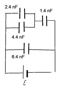
We say that  $C_{\rm eq}$  is the  $\mathit{equivalent}$  capacitance of the two capacitors in parallel.
